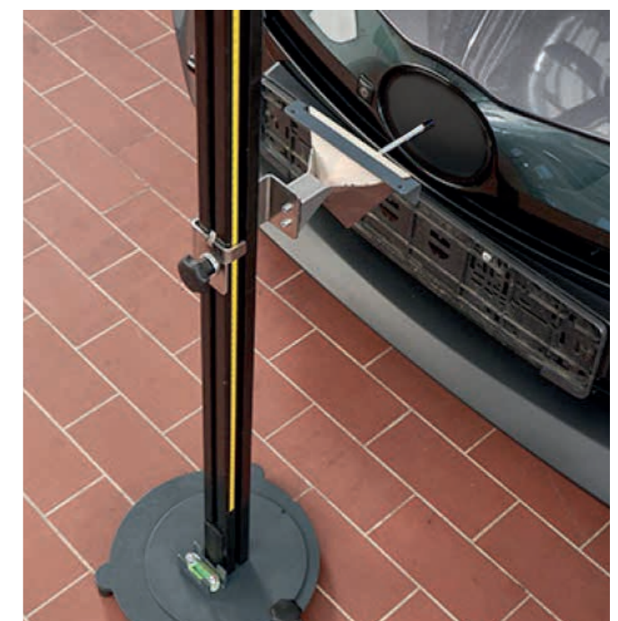
Option to adjust height setting with mechanical indicator pointing on vehicle reference point (emblem)
