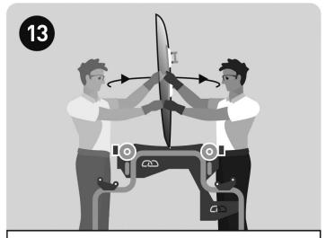
Turn around the table while maintaining the windscreen in a vertical position.
